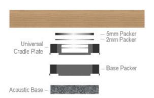
The Durabella Cradle System is designed for applications where the sub-floor is out of level tolerance or uneven and is an extension of the principle applied to the batten system. Durabella Cradle and Batten systems have the ability to resist compression under load whilst providing a continuing level of sound insulation.
